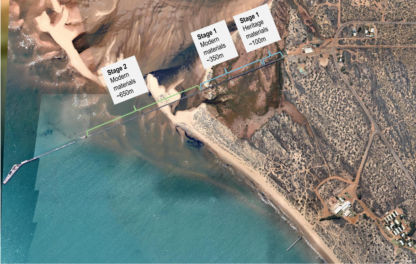
Figure 2: Proposed staging of One Mile Jetty redevelopment
