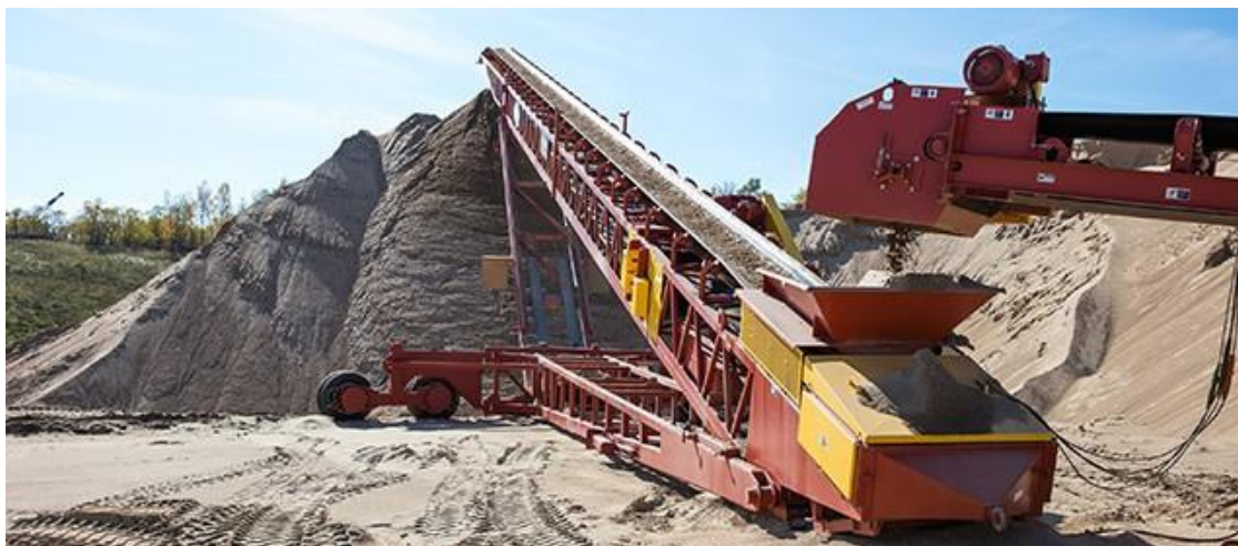
Figure 3.8 Stockpile conveyor (Superior Ind)
